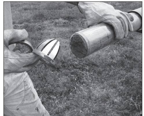
Figure 4.15. Remove liner retainer and core catcher.
