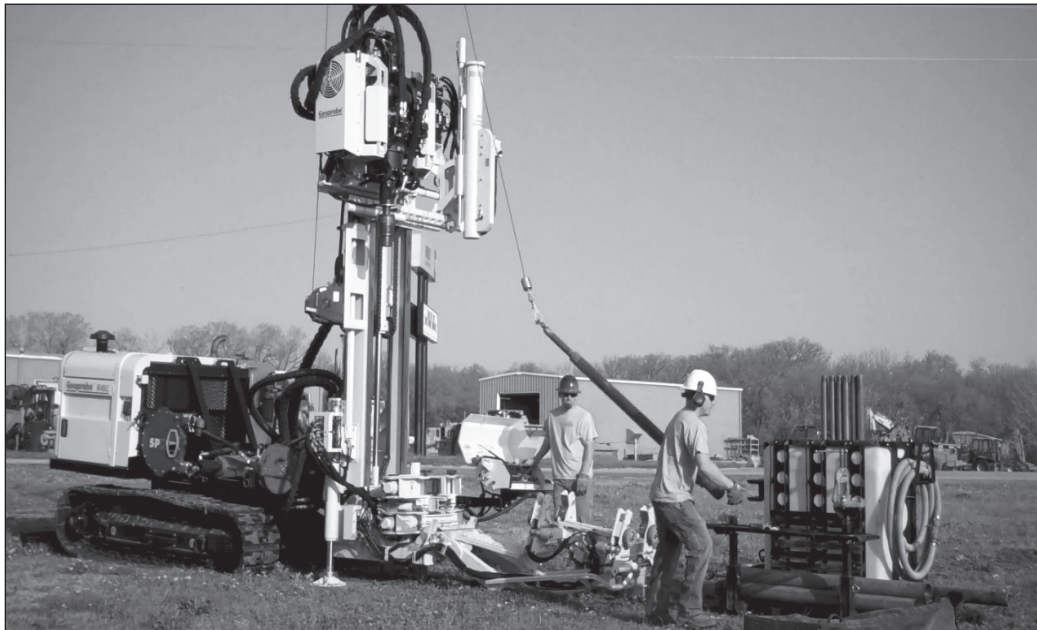
Figure 4.12. Inner rods and sample sheath are retrieved.
