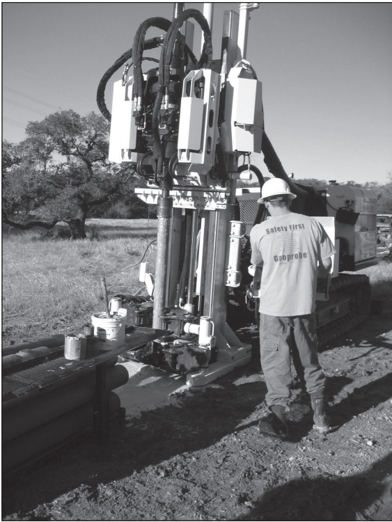
Figure 4.10. Advancing the SDT45 Sampler
