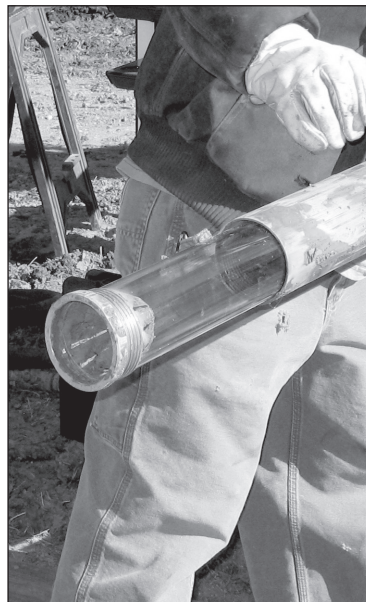
Figure 4.4. Liner, core catcher, and liner retainer are slid into sample sheath.
