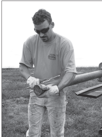
Figure 4.14. The wrench can be used to gently knock off the retainer.
