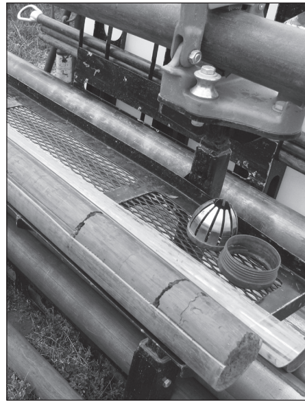
Figure 4.17. Slit liner exposing the sample.
