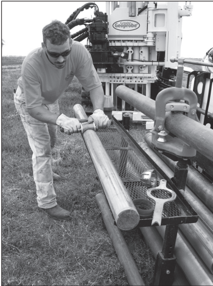
Figure 4.16. Use the SDT45 Liner Cutter to safely expose the sample.
