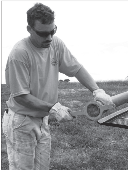
Figure 4.13. Remove the liner retainer with liner retainer wrench.
