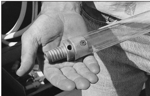
Figure 4.14. Liner attached to liner drive head and ready for sampling.
