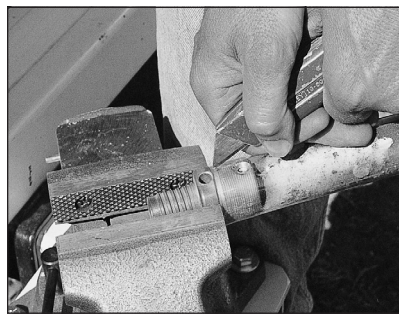
Figure 4.25. Score a line from top of liner to base of liner drive head using a utility knife.
