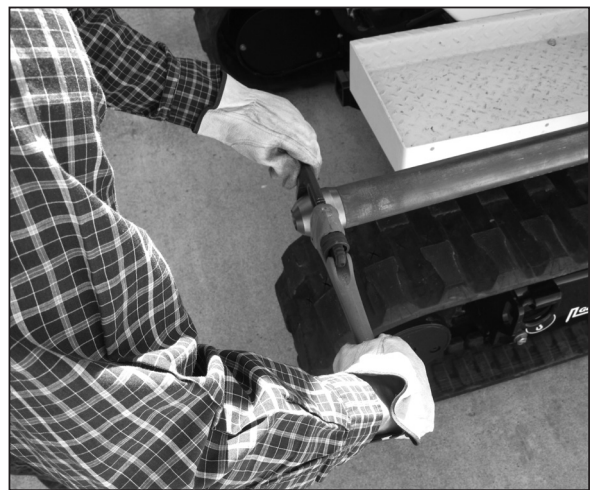
Figure 4.16. Place probe rod (outer casing) in a vise and tighten the cutting shoe with a pipe wrench.
