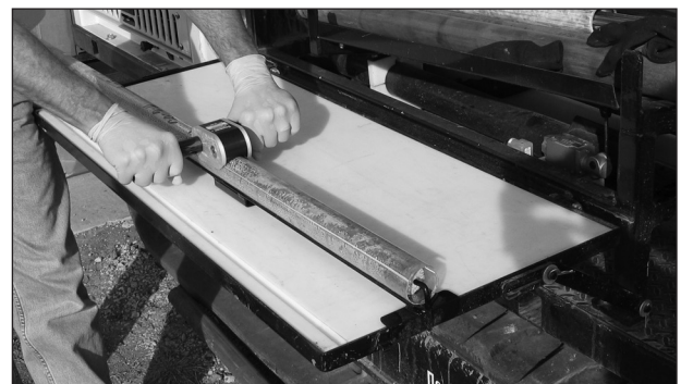
Figure 4.29. Secure the liner with the universal liner holder for cutting. Always place the liner holder on a solid surface such as the work table shown here.
