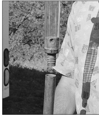
Figure 4.19. Thread liner and liner drive head into 1.25-inch Light-Weight Center Rod.
