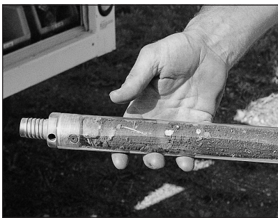
Figure 4.24. Liner drive head remains attached to filled liner after retrieval from outer casing.
