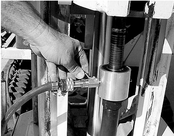
Figure 18. A hose connection, ball valve, and swivel assembly provide water for bit cooling and lubrication.
