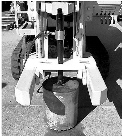
Figure 20. System correctly positioned for coring.
