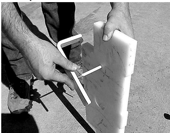
Figure 4. Position bracket as shown and thread onto handle 2 or 3 revolutions.
