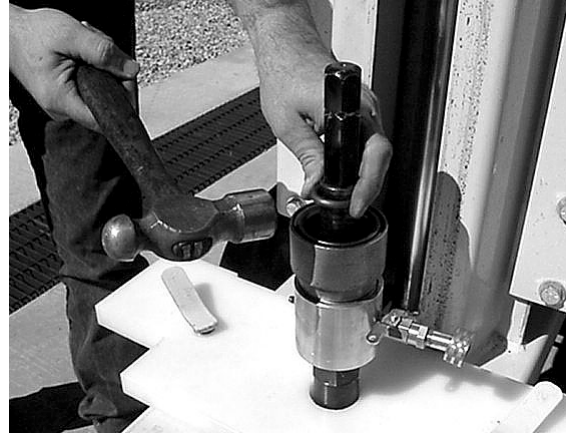
Figure 7. Install a spring clip in the lower groove of the water swivel shaft for GH40-Series applications.
