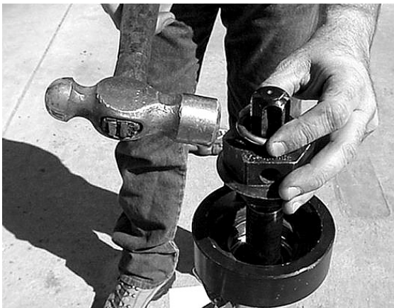
Figure 8. Install a spring clip in the upper groove of the water swivel shaft for GH60 applications.
