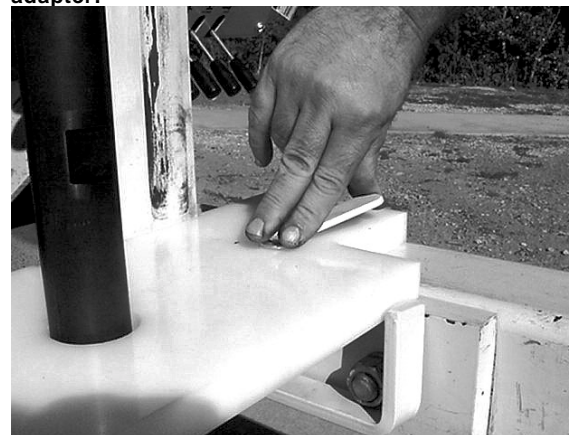
Figure 17. Tighten holding brackets to secure support plate on foot.
