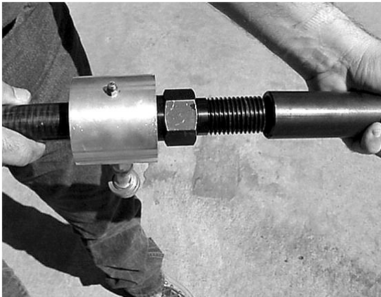
Figure 2. Thread bit extension onto water swivel assembly.
