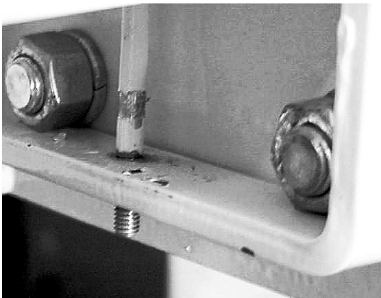
Figure 16. Holding brackets clamp to bolts inside of 6600-Series foot.
