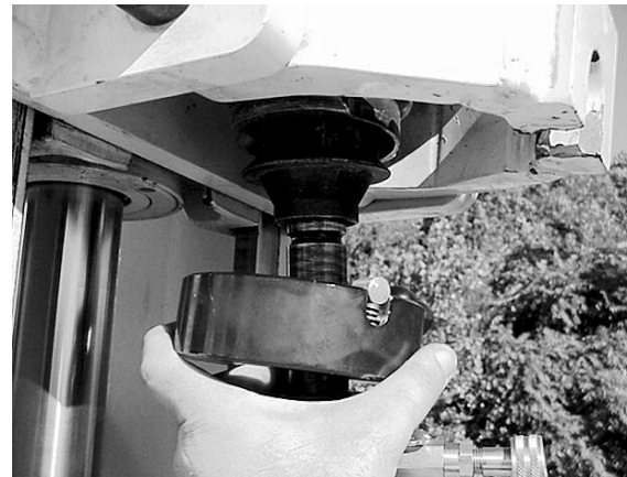
Figure 15. Guide GH60 hex adapter into hex drive while slowly lowering hammer. Keep hand below adapter!
