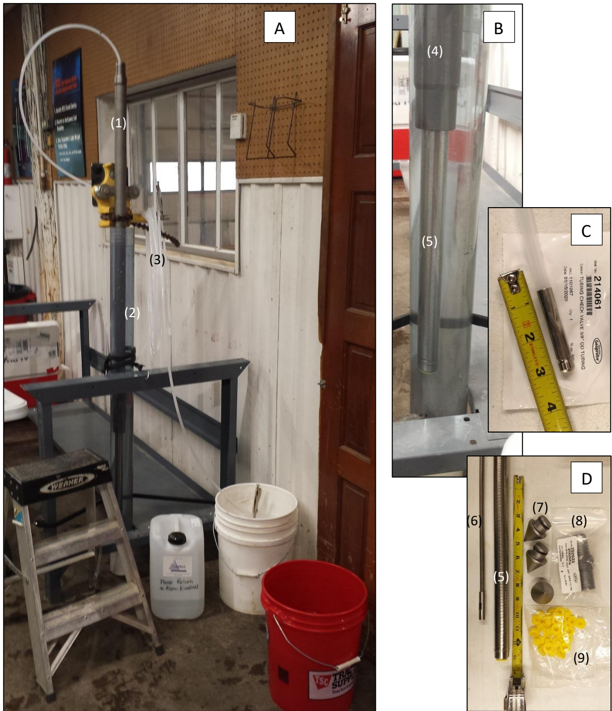
Photograph 1: A) Bench set up of SP16 (1) in 3" clear PVC standpipe (2) with 40 ft of 3/8" LDPE tubing (3) and check valve (not visible) used for purging. B) Screen sheath (4) with 1 ft of exposed stainless steel screen (5) in the PFAS free water-filled standpipe. C) Tubing check valve installed on 3/8" LDPE tubing used for purging/sampling. D) Other components used in the rinsate test include (5) stainless steel screen (6) extension rod with screen push adapter (7) expendable points (8) SP16 drive head and (9) grout plugs.
