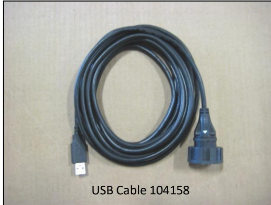
Figure 5: The 15ft USB cable is used to attach the data acquisition module (GW2610) to the laptop computer for signal transmission. The USB cable also provides power from the laptop computer to operate the acquisition module and the transducer downhole. If needed the 12V power inverter (Figure 1, 107479) included with the kit may be attached to the Power Point of a Geoprobe® unit or vehicle to recharge the computer battery.
