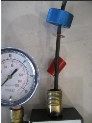
Figure 4: Transducer seal assembly showing the knurled cap, copper washer and split bushing on the transducer cable after the transducer is lowered to depth.
