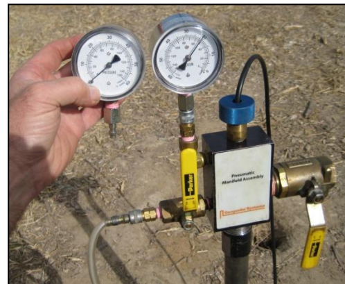
Figure 14: Use the vacuum gauge to perform falling head tests or install the pressure gauge to conduct rising head tests and for leak testing.
