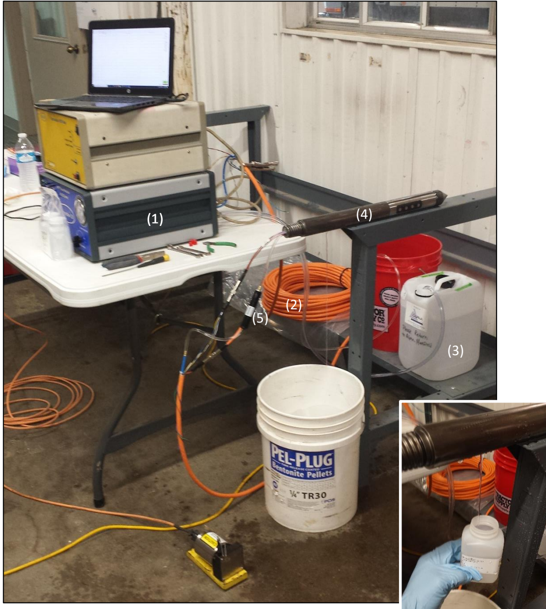
Photograph 1: Bench setup of the HPT system for PFAS rinsate testing. Components include:
