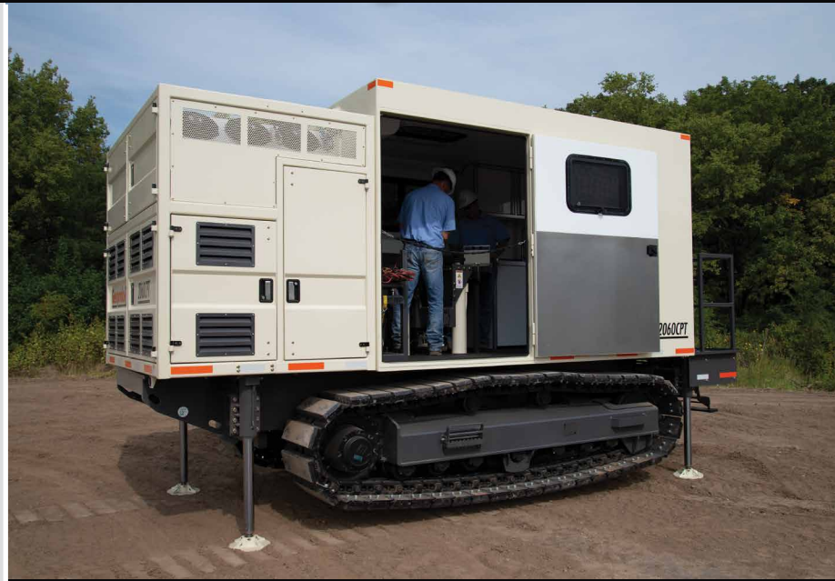
The 2060CPT features 20-tons of downforce and 30-tons pull.
