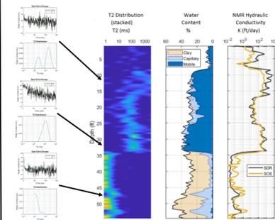
The  $T_2$  distribution is associated with the varying pore size throughout the log from highly permeable, longer relaxation times of sands and gravels in the top 34ft of the log to much quicker relaxation times of silts and clays below 34ft. The varying formation structure can be seen within the spin-echo decay times and  $T_2$  distribution call outs.
