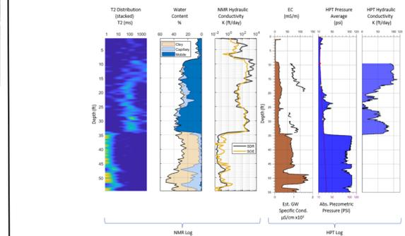
This NMR log was collocated with an HPT log which confirm the static water level at approximately 9ft, a highly permeable aquifer between 8-34ft as well as some silty material between 20-25ft and a couple slightly more permeable zones between 45-55ft. The HPT hydraulic conductivity (K) estimation reaches its model limits of ~75ft/day in the top 7ft of the aquifer and between 30-35ft. The NMR models can effectively estimate K an order of magnitude above and below the HPT estimations.
