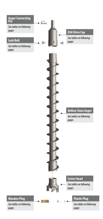
Hollow stem augers can act as temporary casing, keeping the sides of the bore hole from caving in, allowing the crew to take samples through the hollow stem or use it for setting a groundwater monitoring well into place. While not effective when boulders or large cobble stones are encountered, split spoon or continuous coring can be successful in loose, sandy soils.
