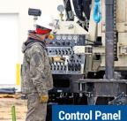
**Durable, mechanical controls** simplify operation and training of new drillers. Organized control panel includes engine monitoring, safety E-stop, hydraulic pressure gauges, friction control levers for mud pump and rotation circuits, and electronic throttle controls.
