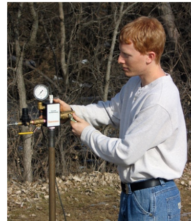
The pneumatic manifold provides the valves, fittings, and gauge (scaled in inches of water) necessary to conduct pneumatic slug tests with Geoprobe® groundwater samplers or wells.
