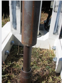
When sampling with the DT22 system, the smaller OD probe rods are placed inside the outer casing and hold a sample liner in place as the outer casing is driven one sampling interval.
